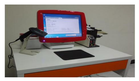
The Station is a staff assisted station on services such as tagging and security operation. This conversion station is used to program RFID tags on new or existing library items. It is helpful when the library moves from barcode to RFID equipment.
