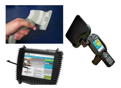
The Shelf Management Solution makes locating and identifying items on the shelves an easy task for librarians. It comprises basically of a portable scanner and a base station.
